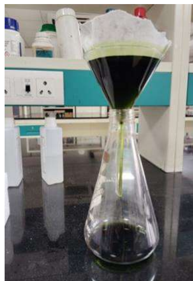
Figure 3 Coarse form of Salix alba crude drug at ambient room temperature with ethanol and distilled water in the ratio of 80:20 in the macerator apparatus. Periodic shaking was done at regular intervals.
