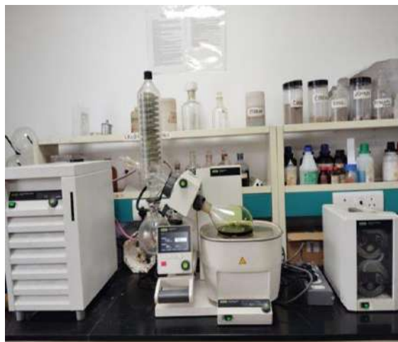
Figure 5. Removal of excess solvent and preparation of Concentrated extract using BUCHI Rotavapor R-300
