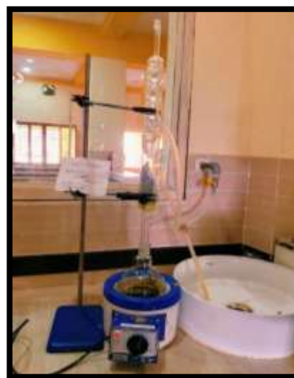
Fig 5: Soxhlet's extraction process of Ocimum sanctum by the solvent ethanol
