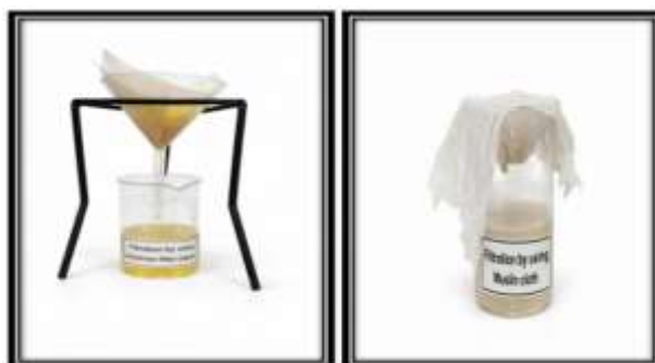
Fig 5: Primary Filtration by Muslin cloth and Secondary Filtration by Whattman filter paper
