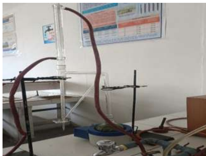
Figure No. 6: Extraction of Essential oil using Clevenger Apparatus
