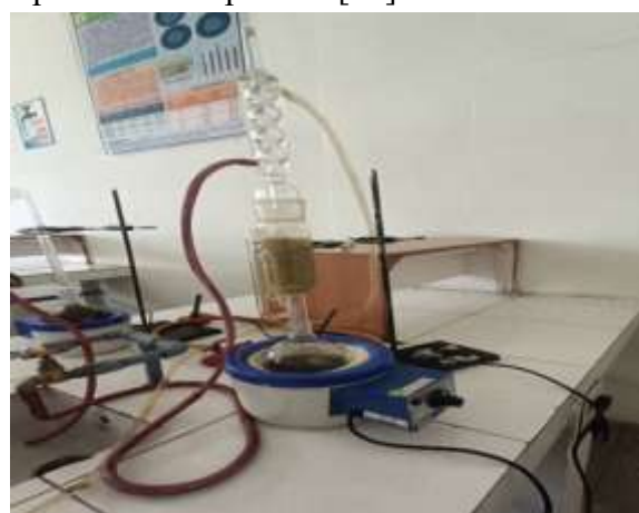
Figure No. 5: Extraction using Soxhlet apparatus by Hot continuous percolation method
