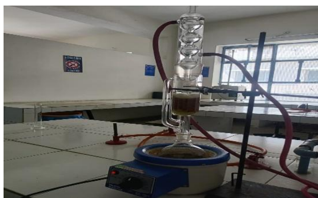
Figure:3 Extraction of ajwain seed by soxhlet extraction
