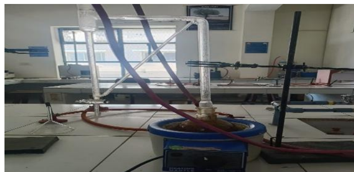
Figure no: 4 Isolation of ajwain oil by Clevenger apparatus.
