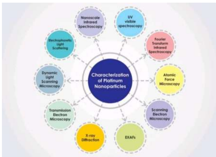
Fig.no 5 : The Different Ways in Which Characterization of Platinum Nanoparticles Can Be Done.
