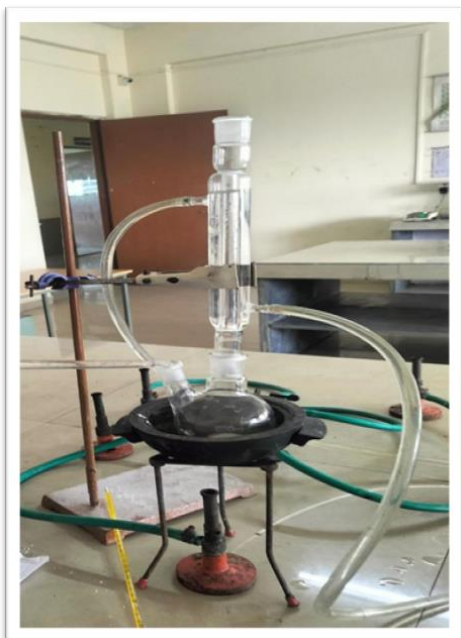
Fig no.3: Reflux condensation of synthesis of methyl 4-sulfamoylbenzoate.
