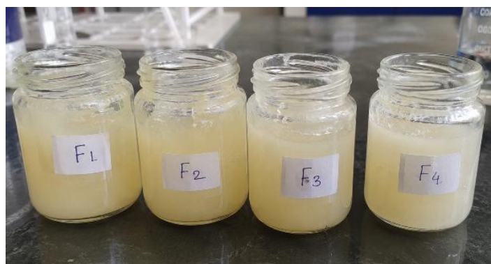
Figure 4. Photograph of the prepared topical gel formulations (F1–F4) containing the synthesized Schiff-base derivative with varying concentrations of Carbopol 940.
