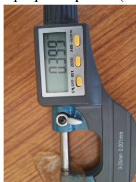
Figure no. 02a measuring the thickness of patch using micrometer
