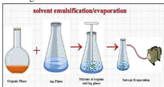
Figure-3: Schematic Diagram of Solvent Emulsification/Evaporation Process involved in Preparation of SLNPs 24
